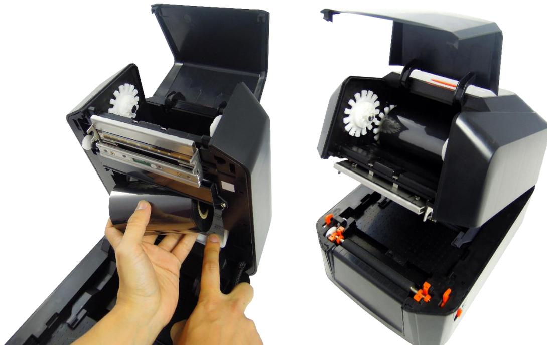
4. Load the right side of paper core first into the ribbon take-up mechanism.
