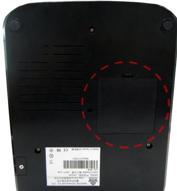
2. Push the button located beside battery as below Figure, the battery will be separated from the motherboard.
