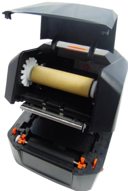
5. Pull the ribbon to bypass print head and then attach the ribbon leader on the empty paper core with tapes, then rotate the ribbon rewind wheel until ribbon surface has no wrinkle; Close the ribbon cover to finish ribbon installation.
