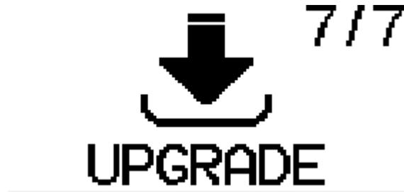
Place the updated firmware in the WPL\_Stuff folder of SD card, and take this SD card inserting to the printer, then use this Upgrade option to click the selected file to confirm the updated procedure.
