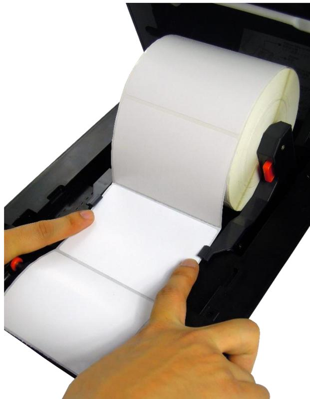
2. Pull the label paper through the rubber roller and push the both sides of label under the label guides. Close the top cover to finish label installation.
