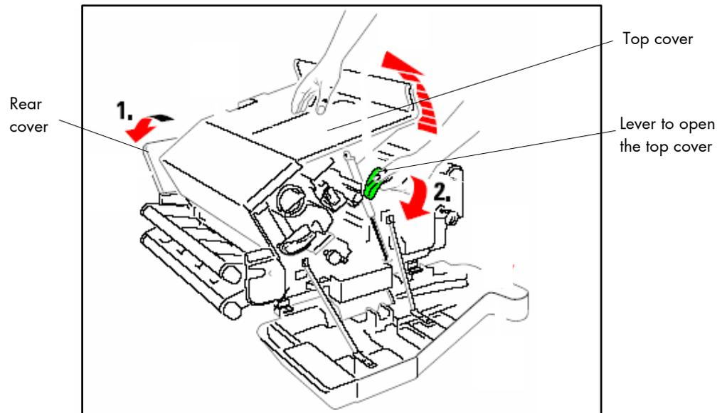
Fig. 2.4.4.a Opening the rear and top cover
