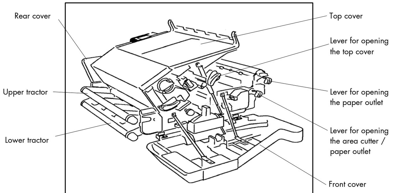
Fig. 8.4.4.d **Overview:** Printer SOLID 33E-2 / 58E opened
