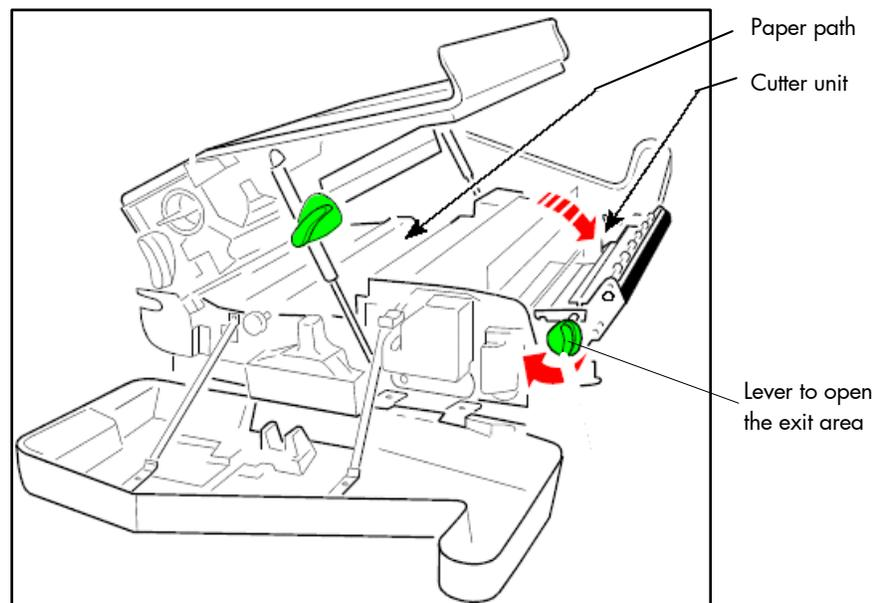
Fig. 7.1.2.e Opening the paper exit area
