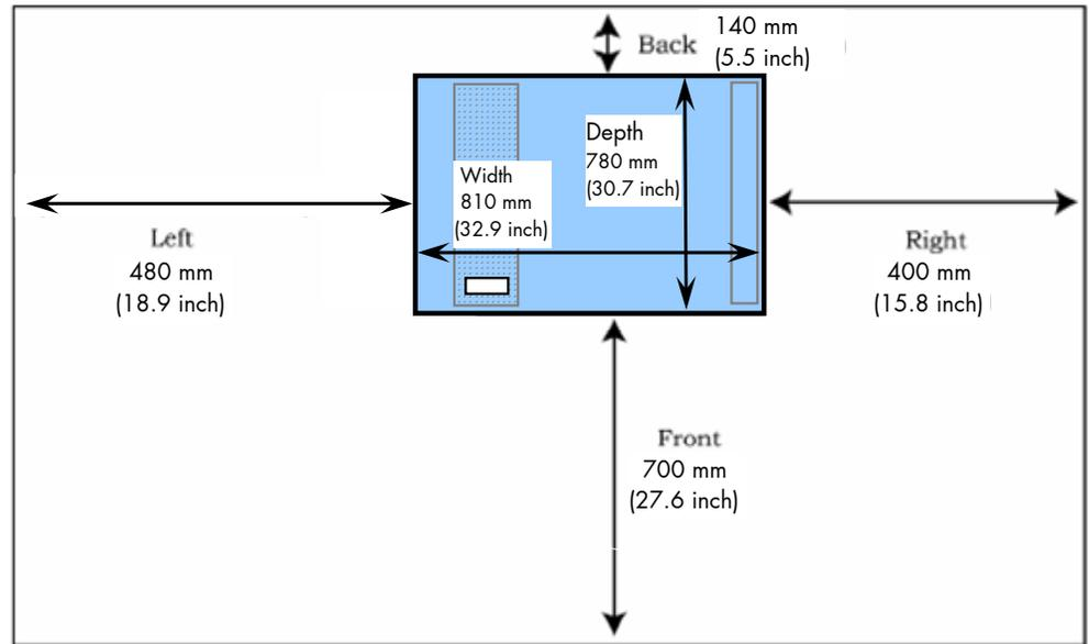
Fig. 2.3.a SOLID 33E-2 and SOLID 58E: Required space (plan view)
