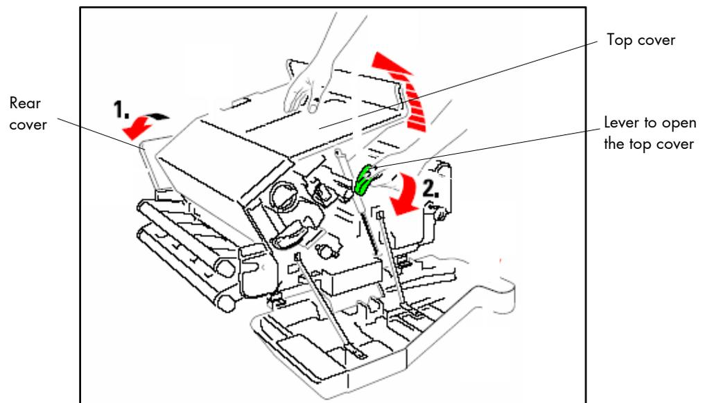
Fig. 7.3.a Opening the rear and top cover
