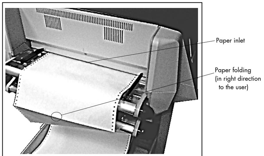
Fig. 4.1.2.d Paper inserting
