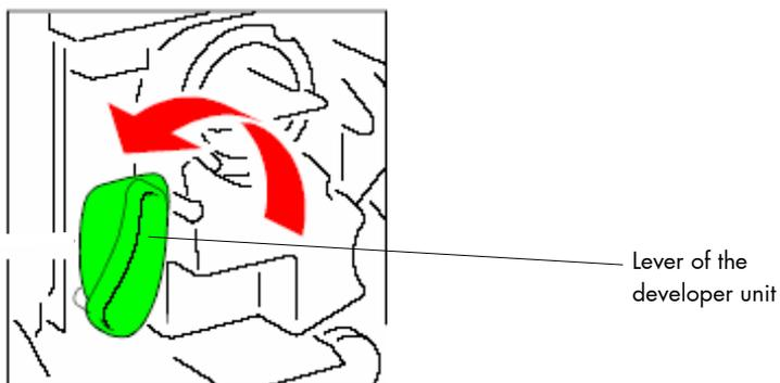
Fig. 7.1.2.b Detail: Unlocking the developer unit
