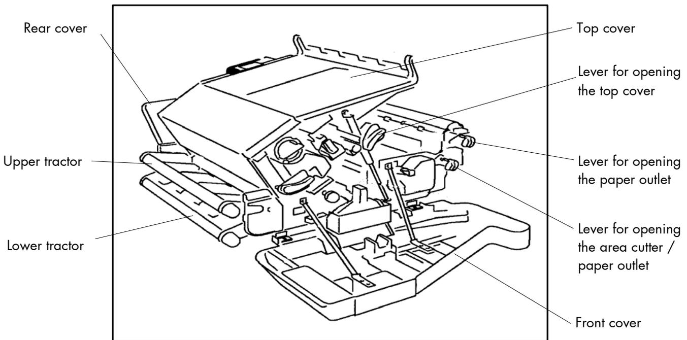
Fig. 2.2.d Printer SOLID 33E-2 / 58E opened
