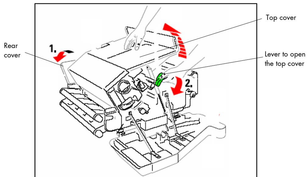
Fig. 7.4.a Opening the rear and top cover
