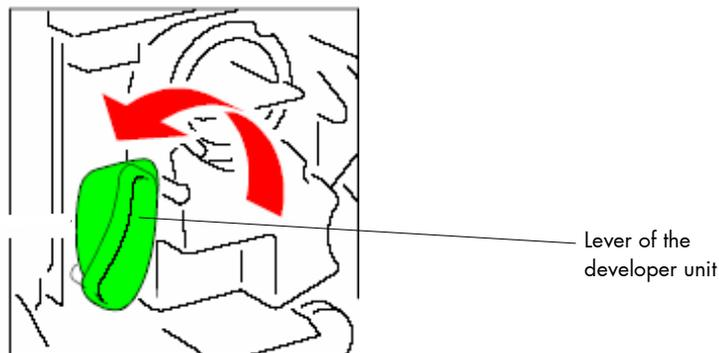
Fig. 2.4.2.b Detail: Unlocking the developer unit
