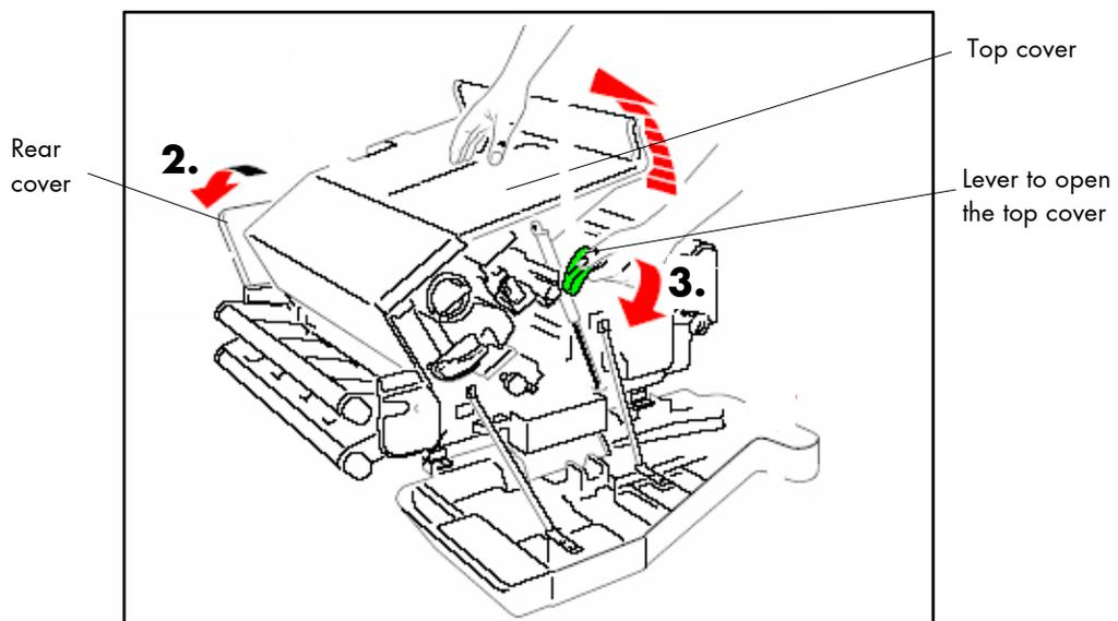
Fig.8 4.4.b Opening the rear and top cover
