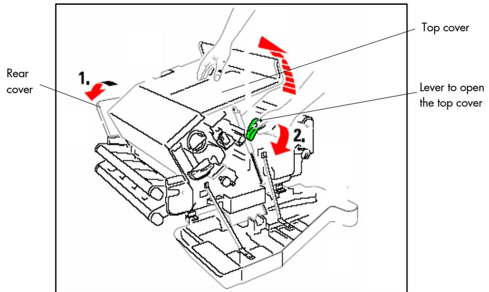
Fig. 7.1.2.d Opening the rear and top cover
