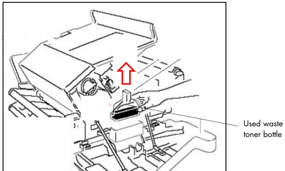
Fig. 7.3.b Removing the used waste toner bottle
