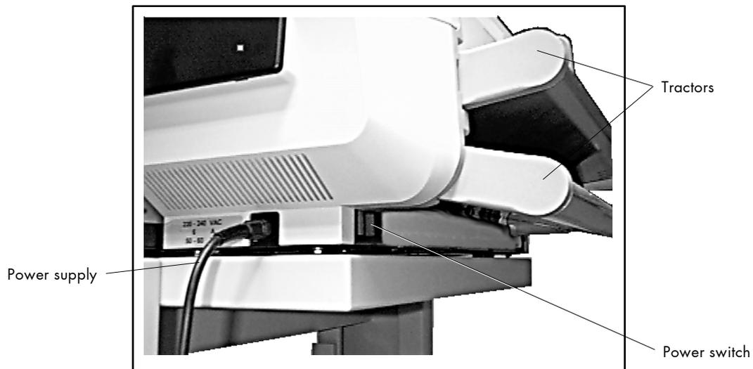
Fig. 5.2.a Turning on the printer (printer's rear view)
