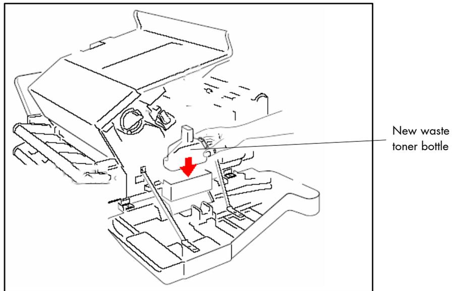
Fig. 7.3.d Installing the new waste toner bottle
