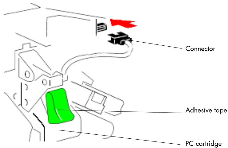
Fig. 2.4.7.b Attaching the electrical connector
