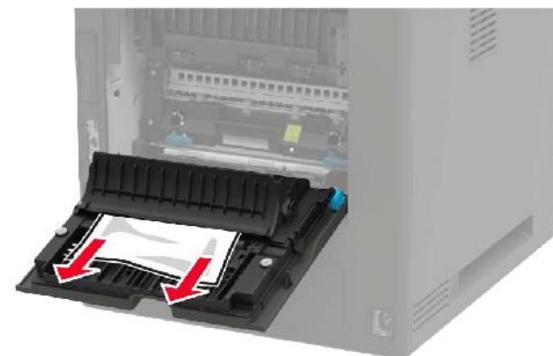
Fig. 11.4.5.d Removing jammed paper from the duplex area
