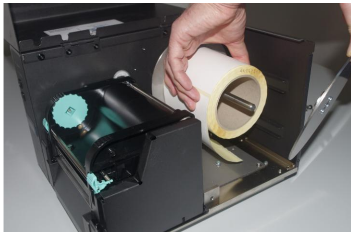
Fig. 4.3.1.h Holding the media roll and taking the front spacer
