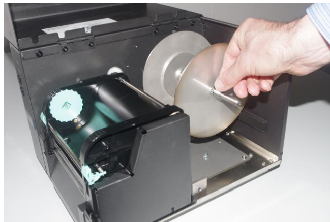
Fig. 4.3.1.c Loosening the front knurled screw
