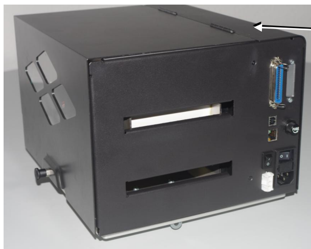
Fig. 5.2.a Rear view of the printer: Position of the side cover
