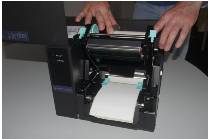
Fig. 4.3.1.s Lateral movement of "all" parts together (i.e.: Media roll together with the spacers and the centering sleeve)
