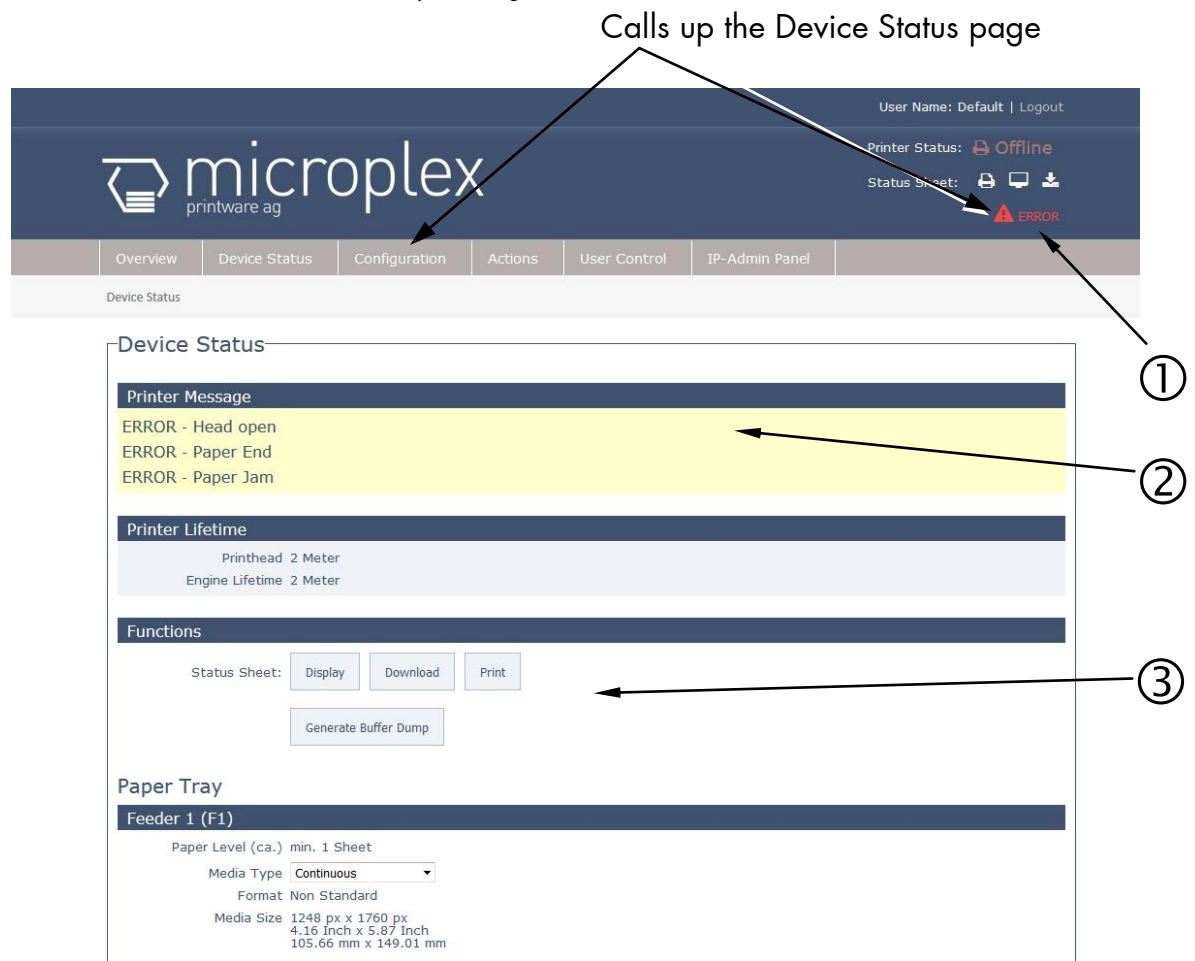
Fig. 7.5.a logiJET TM4: Device Status page of the MICROPLEX WebPanel
