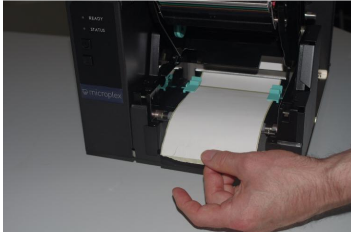
Fig. 4.3.1.p Free end of the media roll pulled out of the printer
