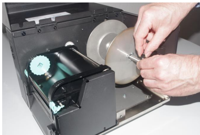
Fig. 4.3.1.d Removing the front centering sleeve
