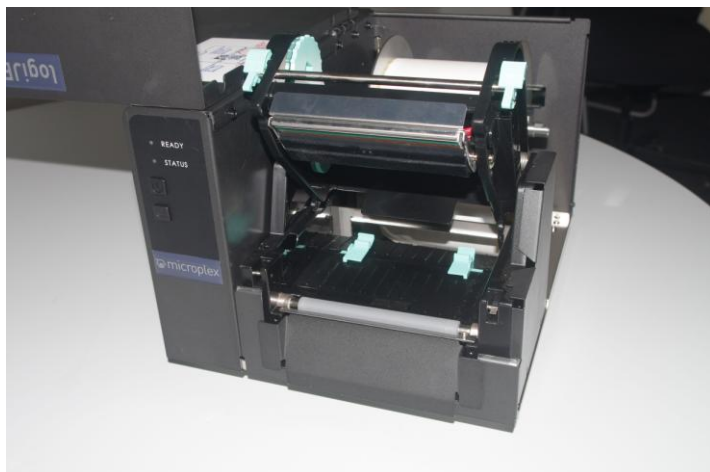
Fig. 4.3.1.m Printhead mechanism swivelled upwards
