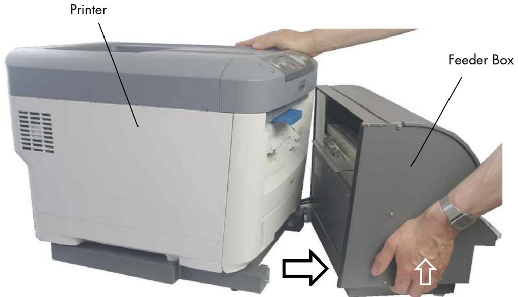
Fig. 7.b Swivelling the Feeder Box away from the printer
