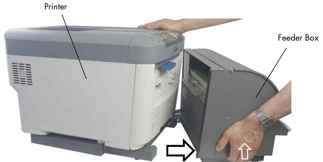
Fig. 6.1.a Swivelling the Feeder Box away from the printer
