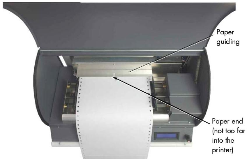
Fig. 3.3.2.1.e Inserting the paper
