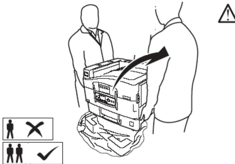
Fig. 2.1.a Lifting the printer
