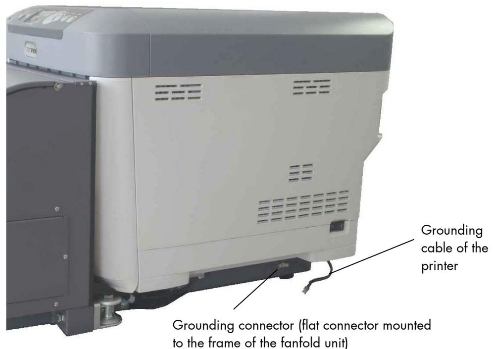
Fig. 2.5.b Grounding cable of the Printer
