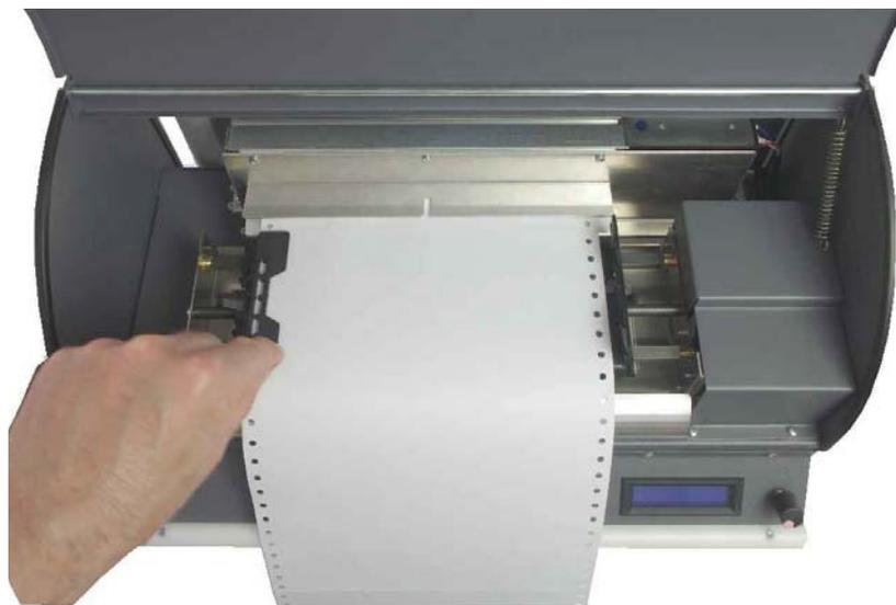
Fig. 3.3.2.1.g Closing the tractor cover plates
