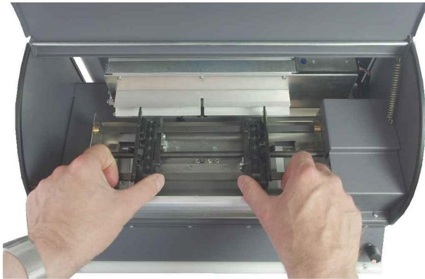
Fig. 3.3.2.1.d Adjusting the tractor to the width of the media to print on
