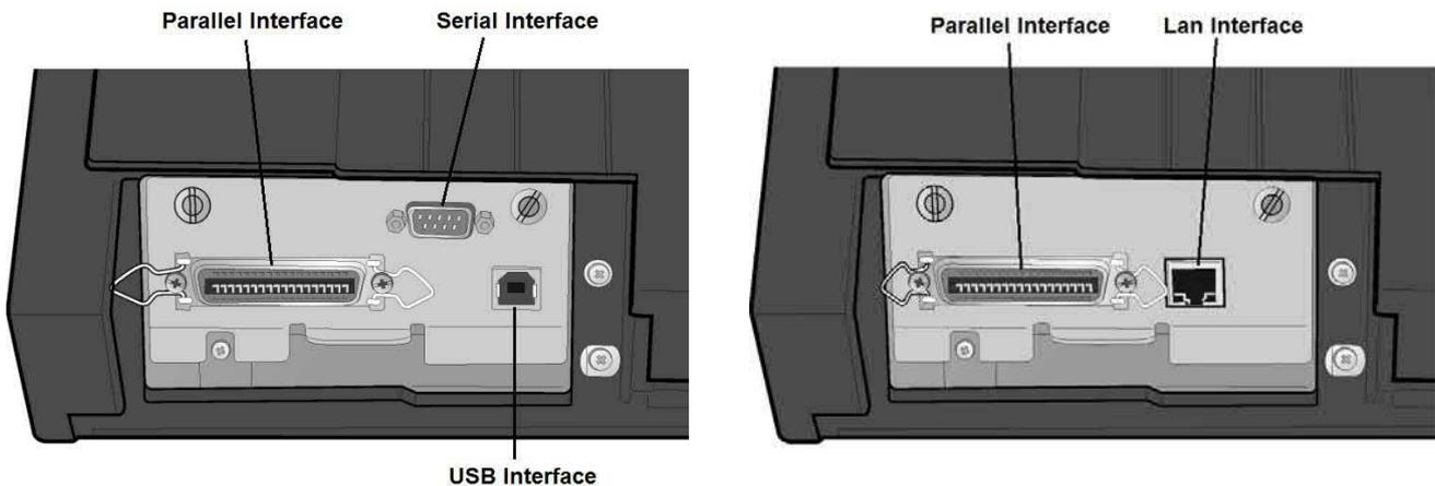
Insert the *parallel interface cable* into the parallel connector and fasten it by means of the clips.
