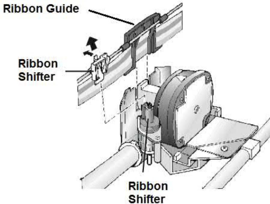
3. Remove the used ribbon cartridge by lifting it up.
