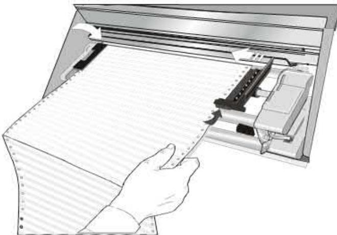
7. Position the left sprocket for printing, matching the left paper margin with the ninth notch on the printer cabinet and lock it in place
