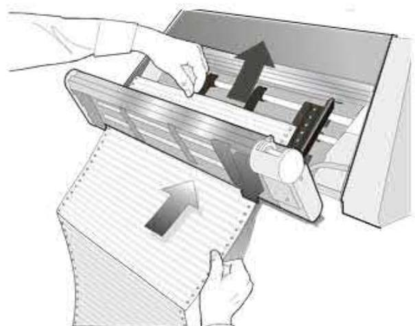
3. When the fanfold paper has been loaded on the Front1 push tractor, reposition the Front2 push tractor in its initial position before closing the Push tractors cover
