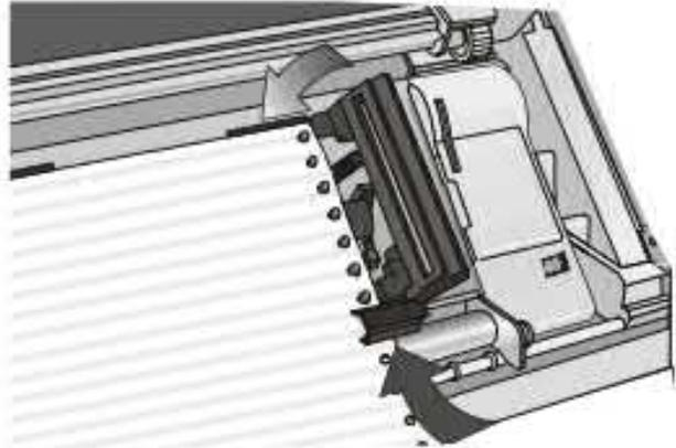
7. Match the left sprocket for the first printing position, i.e. the left paper margin must match the ninth mark on the printer cabinet.
