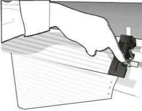
9. Close the Push tractors cover. Press the LOAD/FF key to load the paper into the printer.
