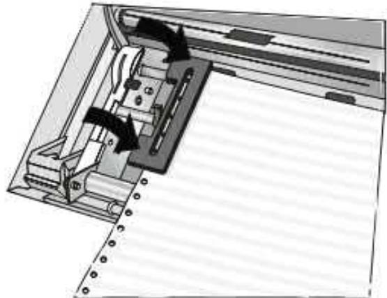
5. Insert the paper on the right sprocket pins and close the right sprocket cover
