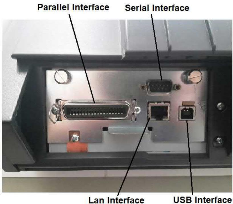
The 9050 printer can be connected to your host computer via different available interfaces on two alternative controllers.
