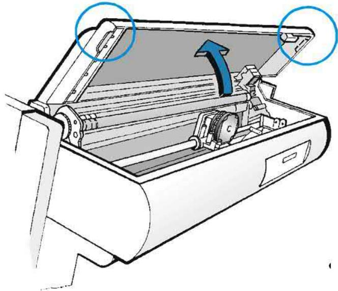
6. Move the print carriage in the middle of the area to prepare it for ribbon cartridge installation
