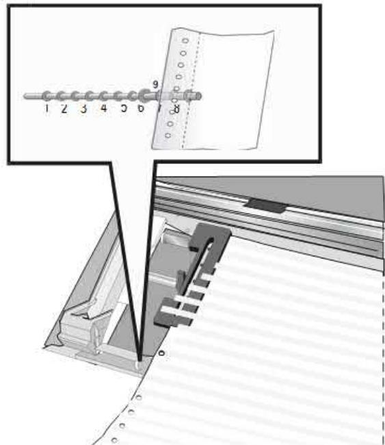
8. Adjust gently the right sprocket to remove slack from the paper. Lock the Front2 tractor sprockets moving the sprocket levers down.
