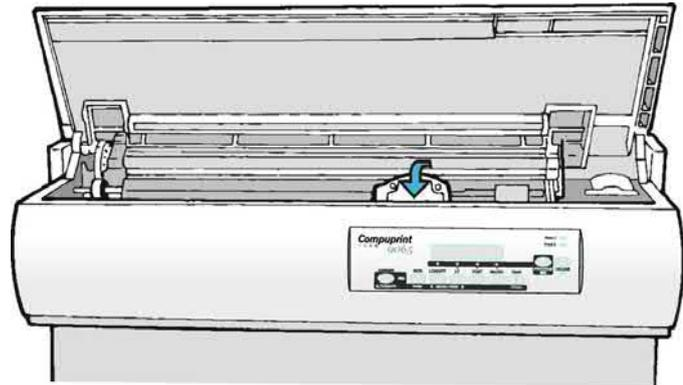
7. Before installing the ribbon cartridge turn the ribbon-winding knob in the arrow direction (located on the cartridge) to take up slack in the ribbon
