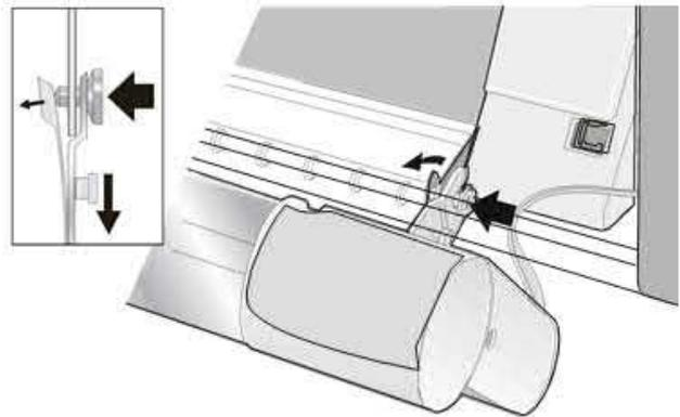
3. Insert the connector cable in the electrical connector located in the lower push tractor
