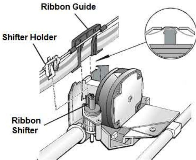
9. Insert the shifter holder onto the ribbon shifter as shown in the following figure.
