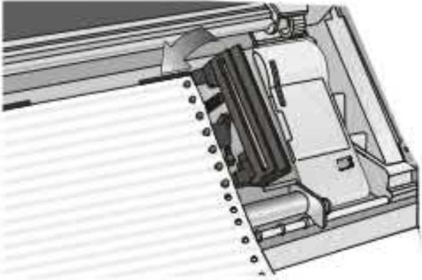
6. If you are using the 6 pin Front1 Push tractor option, make sure the paper goes under the paper sensor, and close the right sprocket cover.
