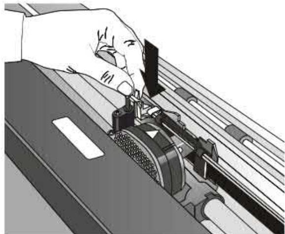
10. Turn the ribbon-winding knob in the arrow direction (located on the cartridge) to take up slack in the ribbon.
