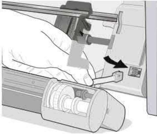
4. Rotate the Front2 push tractor onto the Front1 push tractor.
