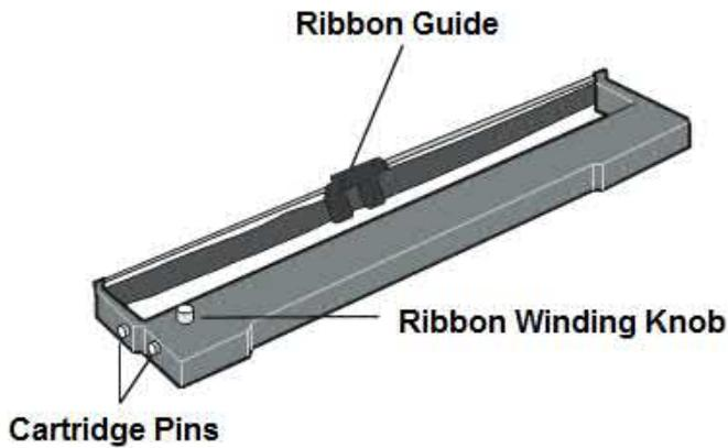
To be used when the ribbon shifter option is not installed
