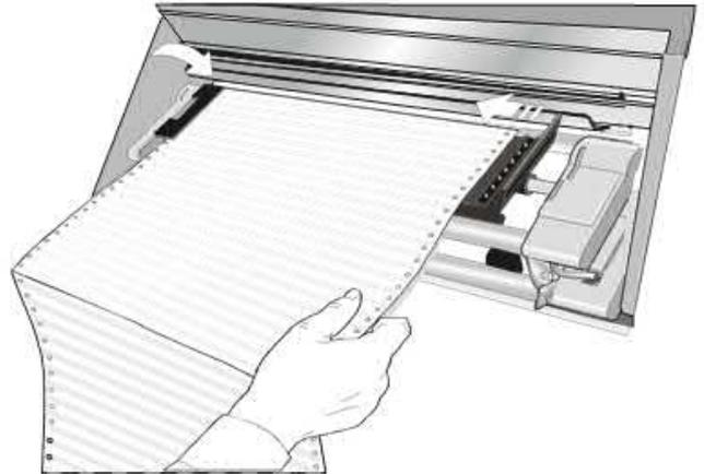
6. If you are using the 6 pin Front2 push tractor option, make sure the paper goes under the paper sensor and close the sprocket cover.
