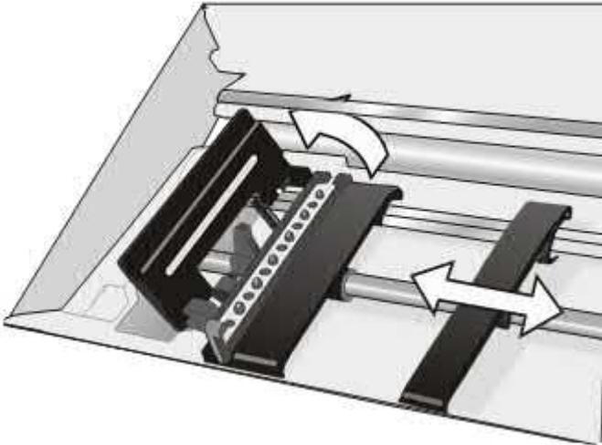
5. Hold the fanfold paper in front of the sprockets and insert the paper perforation on the left sprocket pins and close the sprocket cover. Insert the paper on the right sprocket pins and close the sprocket cover.
