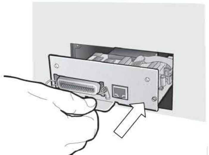
6. Attach the Controller Board with the two screws using the screwdriver that came in the Controller Board box.
