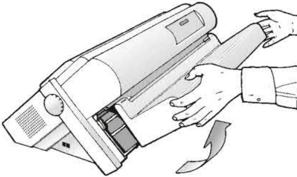
2. Unlock the sprockets of the Front1 tractor moving the sprocket levers down. Slide the left sprocket to the first printing column.
