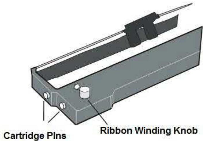
**To avoid damage to the ribbon, do not turn the winding knob in the wrong direction**
