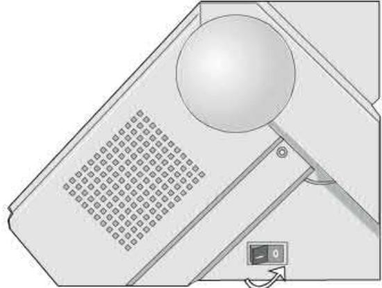
3. Insert the power cable plug into the printer connector and the other power cable end into a convenient outlet (the figure shows the European version).
