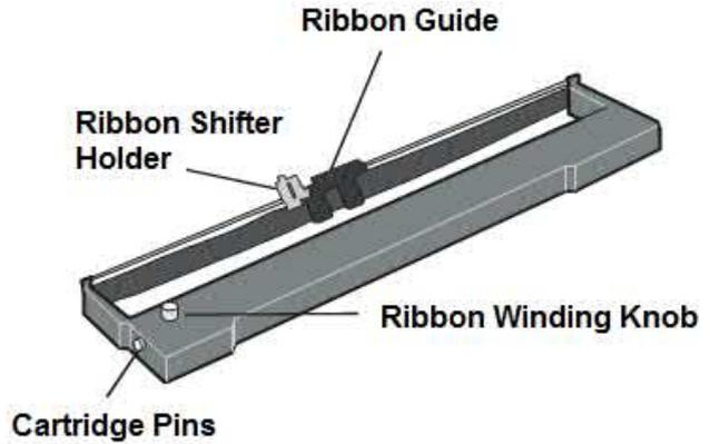
To be used when the ribbon shifter option is installed (see later on for installation of this option)
