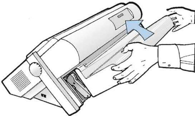
3. Unlock the Front2 push tractor sprockets moving the sprocket levers up
