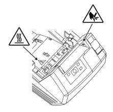
THESE LABELS INDICATE THE RISK OF ANY INJURY DUE TO "HIGHTEMPERATURE" OF THE PRINT HEAD AND "SAW-TOOTHED EDGE" OF THE MANUAL CUTTER.
